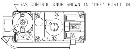
NOTE: Knob cannot be turned from "PILOT" to "OFF" unless knob is pushed in slightly. Do not force.
