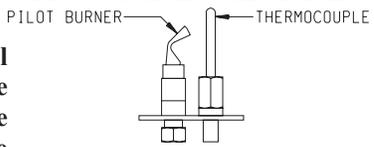
10. Push and hold red reset button down completely and repeatedly push the ignitor button until the pilot burner is lit. Pilot may also be lit with a match. Continue to hold the red reset button down for about one (1) minute after the pilot is lit. Release button and it will pop back up. Pilot should remain lit. If it goes out, repeat steps 5 through 10.
