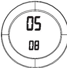
2. Use the ON / s button to set the desired On Delay Time from 0 to 15 min.
