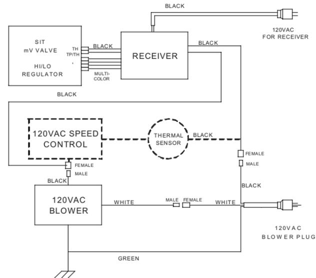
Connect the 30" long 18AWG wires labeled "120VAC FAN ONLY" between receiver and blower as shown in the following diagram as well.
