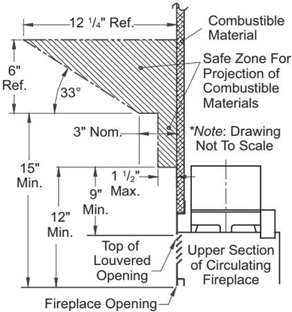
**Figure 4 - Mantel Clearances to Combustible Material (with Louver)**
