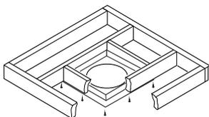
**Figure 13 - Firestop Spacer with Living Space Above Ceiling**
