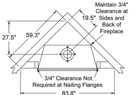
Figure 2 - Corner Installation
