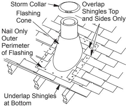
Figure 16 - Flashing Installation
