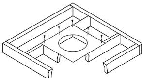
**Figure 14 - Firestop Spacer with Attic Space Above Ceiling**
