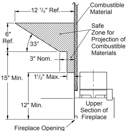
**Figure 5 - Mantel Clearances to Combustible Material (without Louver)**
