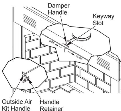
**Figure 25 - Damper and Air Kit Handle**
